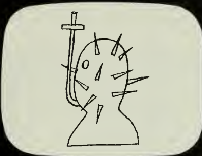
DA VINCI'S leather underwater mask with rigid hoop reinforcement and breathing tube was along right track.
